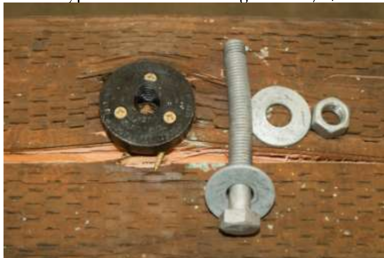
Figure B10. Typical Failure for Configuration3, 5/8-inch Bolt.
