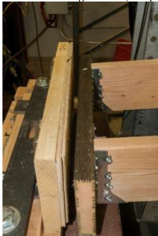
Figure B16. Typical Failure for Configuration 5, Simpson SST Ledger Screw
