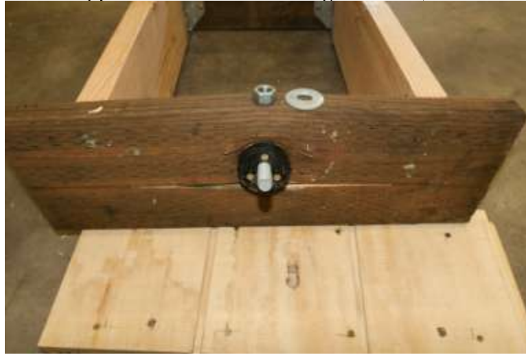
Figure B9. Typical Failure for Configuration3, 5/8-inch Bolt.
