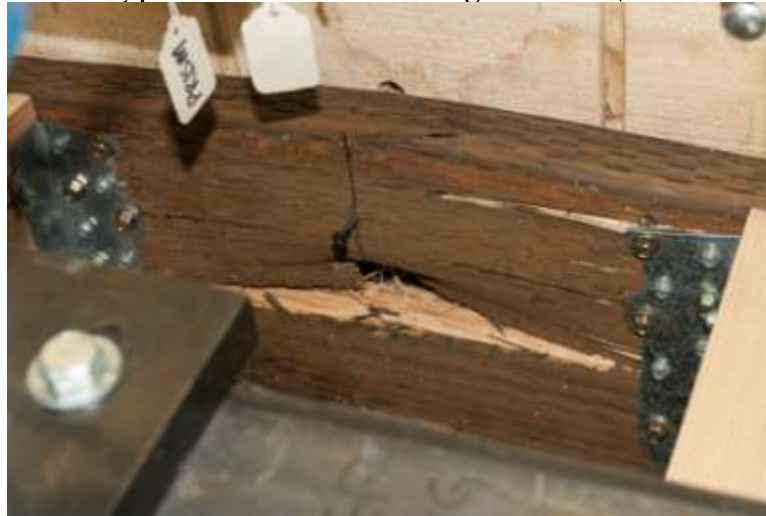
Figure B3. Typical Failure for Configuration 1, 1/2-inch Bolt.
