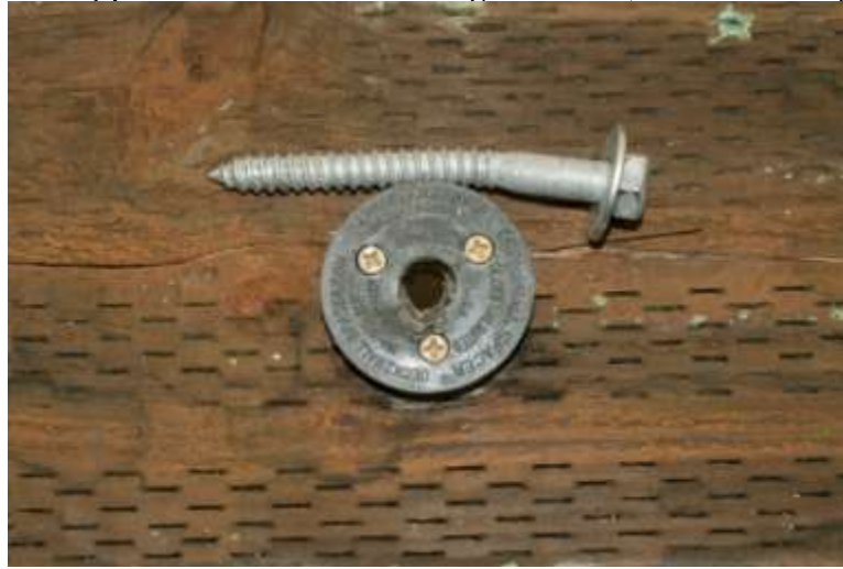
Figure B6. Typical Failure for Configuration2, 1/2-inch Lag Screw.
