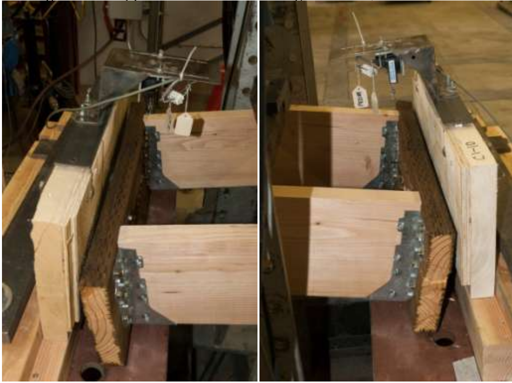
Figure B3. Typical Failure for Configuration 1, 1/2-inch Bolt.
