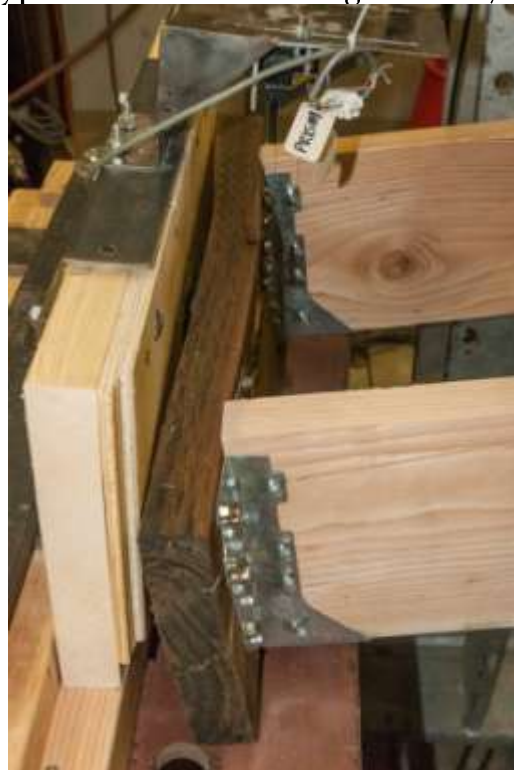
Figure B7. Typical Failure for Configuration3, 5/8-inch Bolt.
