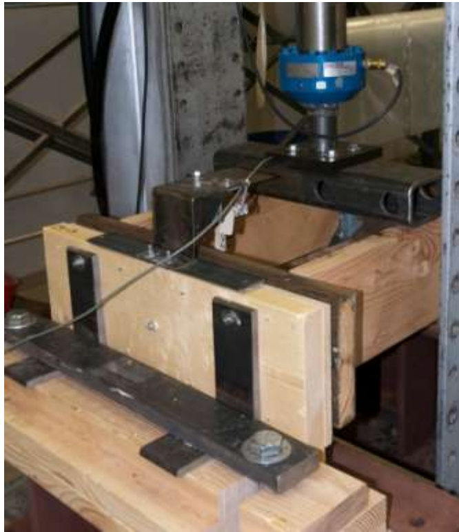
Figure 2. Typical Ledger Testing Specimen with Incised Hem-Fir Ledger Attached Using a \frac{1}{2} - Inch Diameter Lag Screw.
