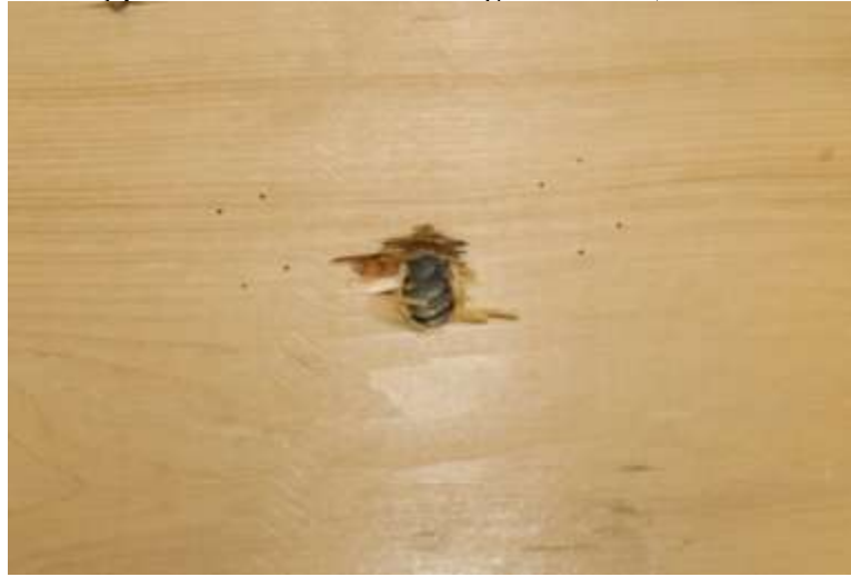
Figure B15. Typical Failure for Configuration 4, 5/8-inch Lag Screw
