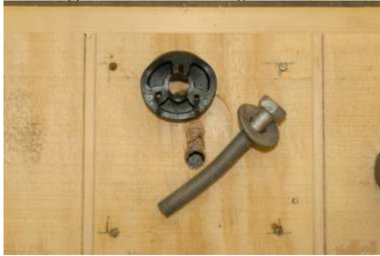
Figure B11. Typical Failure for Configuration 3, 5/8-inch Bolt.
