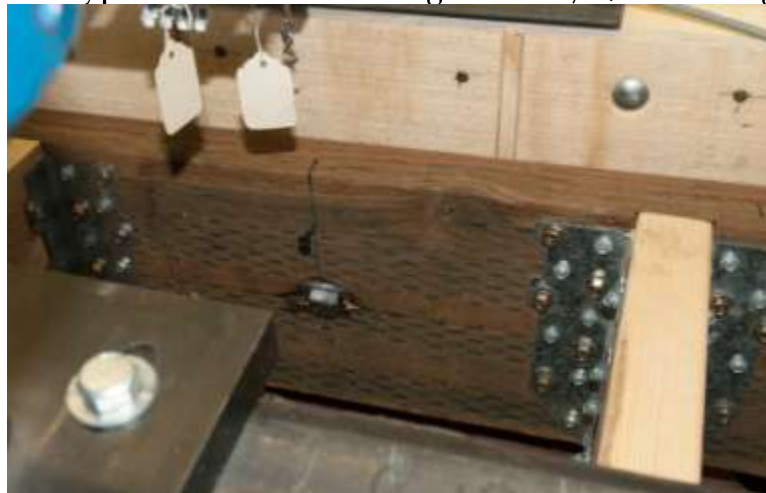
Figure B5. Typical Failure for Configuration2, 1/2-inch Lag Screw.
