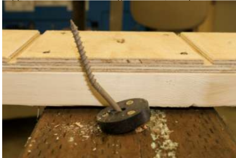
Figure B18. Typical Failure for Configuration 5, Simpson SST Ledger Screw
