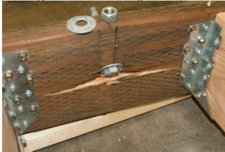
Figure B10. Typical Failure for Configuration3, 5/8-inch Bolt.
