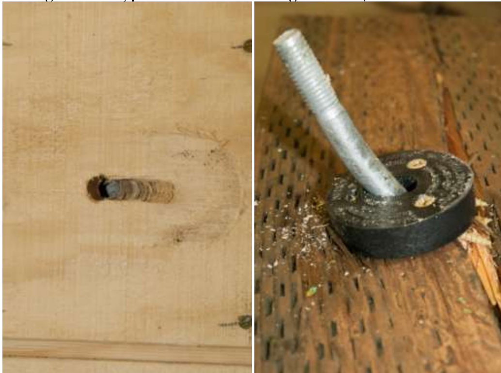
Figure B1. Typical Failure for Configuration 1, 1/2-inch Bolt.
