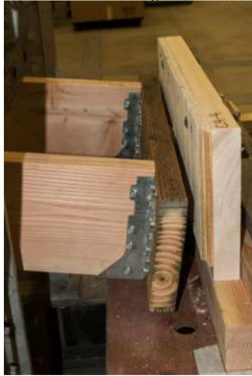
Figure B13. Typical Failure for Configuration 4, 5/8-inch Lag Screw
