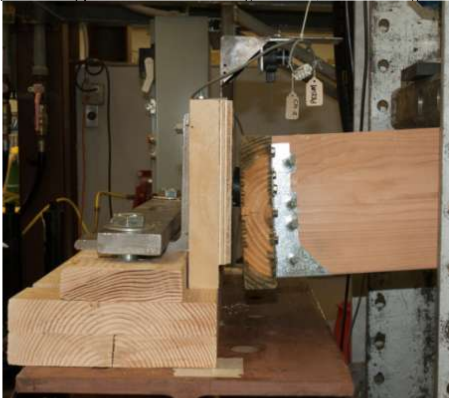
Figure B4. Typical Failure for Configuration2, 1/2-inch Lag Screw.
